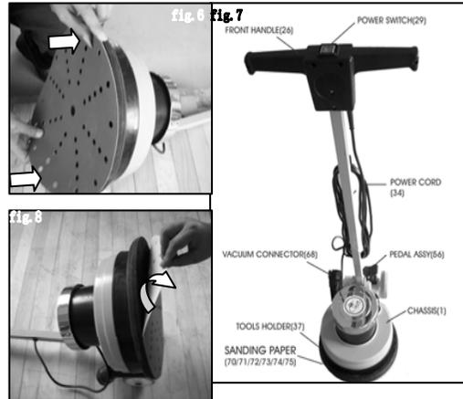
**Replace:** Follow the indication as below to lay the machine on floor, remove the Sanding Paper by hand, as shown on Fig.8, and then replace
